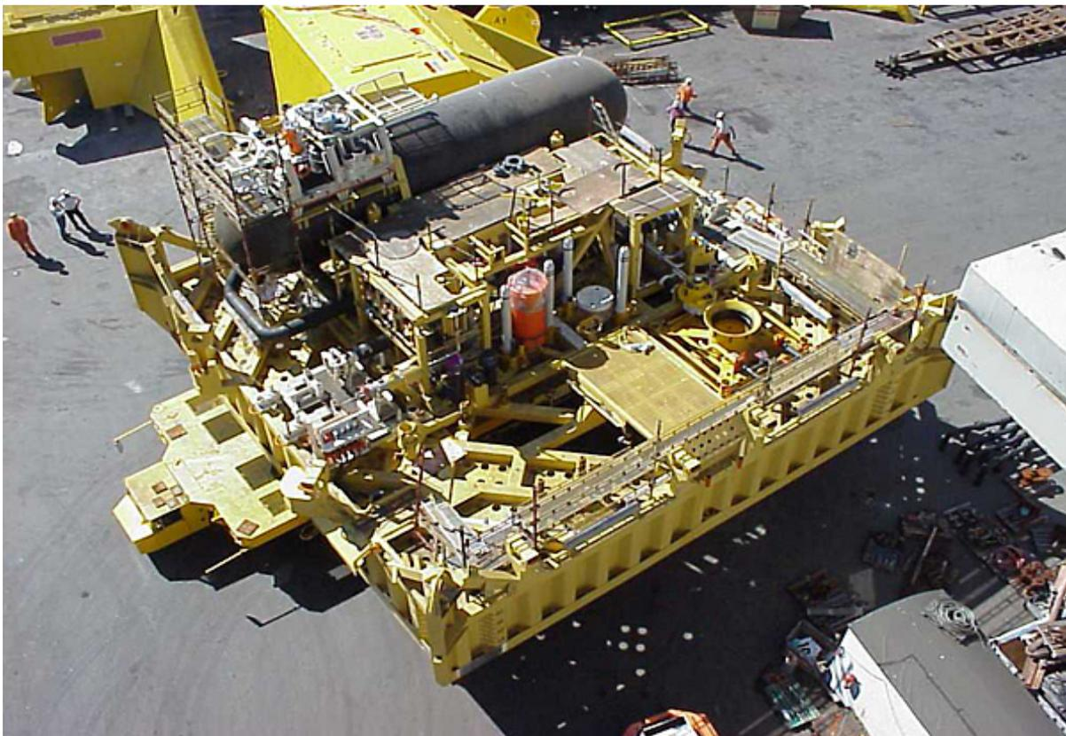
Fig. 3. Seafloor separator on the docks. Note humans above left and right for size
