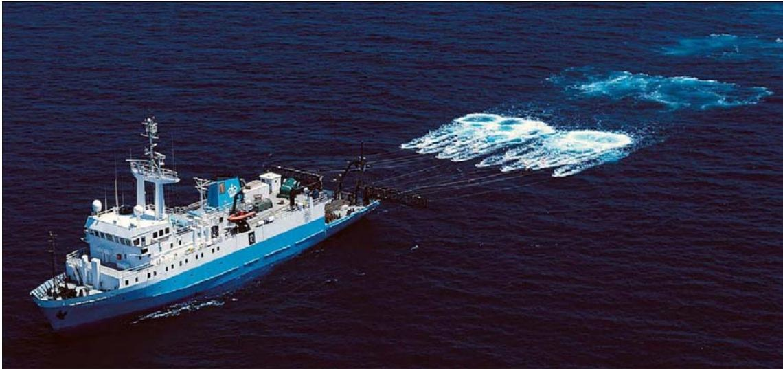
Fig. 1 Towed Airgun Array
