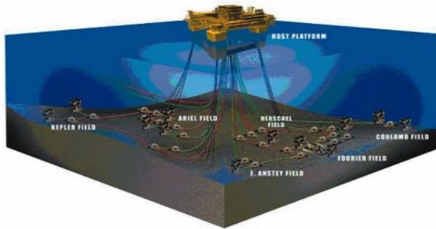
Fig. 2 Multiple oil fields served by a single platform
