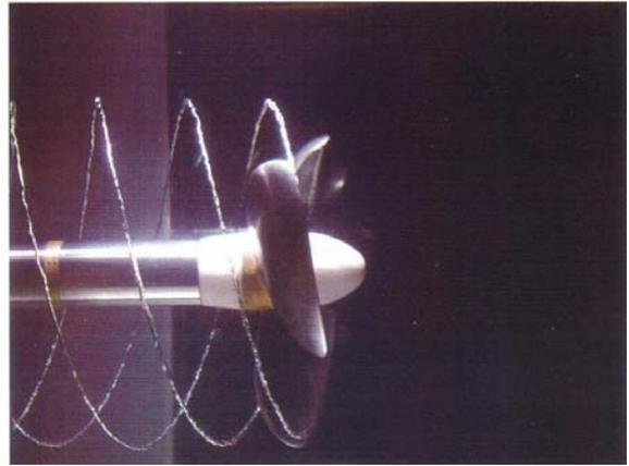
Turbulence from a three blade Pax propeller.
