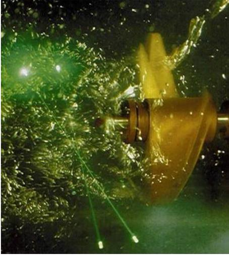
Turbulence from a standard three blade propeller
